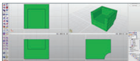
1 Basic form created using two cube primitives and a Boolean operation
